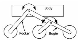
Fig. 3: The "rocker-bogie" concept
