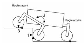
Fig. 9: Forces on the wheels of the rover
