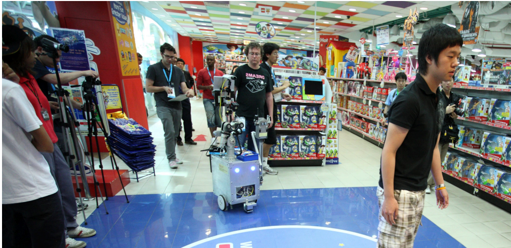
Fig. 19 Robot HR-Y follows a team member, learning, in a first phase, how to get to the shelves where some objects that the referees defined are displayed. In the next phase, the robot is expected to again find the shelf on his own, moving to pick only one object as specified by referees and finally bringing it to the exit.
