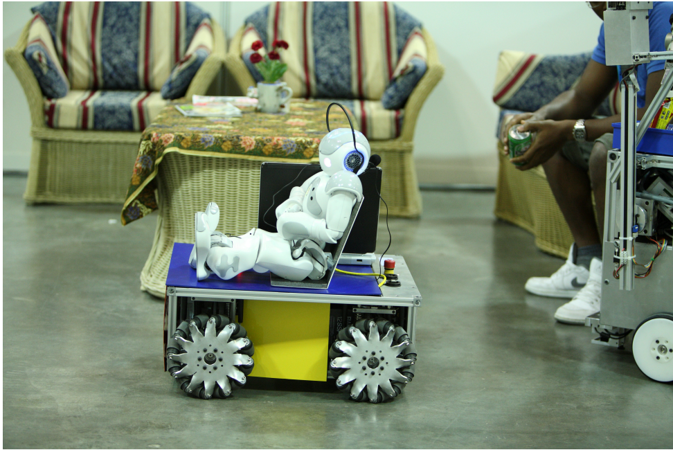
Fig.18 Detailed view of the mediating robot. On this picture, Nono wears an external microphone in order to broadcast his speech on the public facilities.
