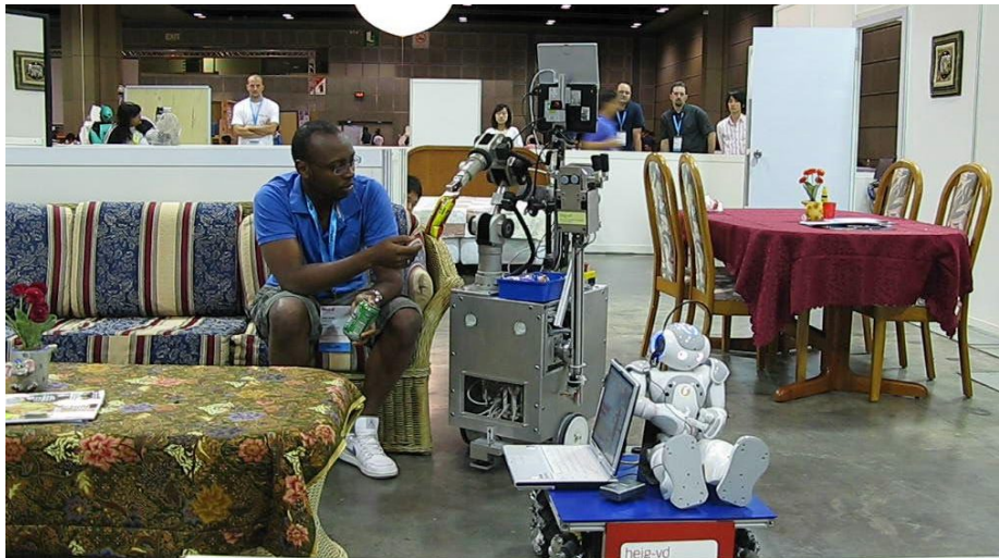
Fig.17 Nono, a humanoid of Nao type (lower right) mediates between humans and other machines. OP-Y is the platform on which Nono is installed; RH-Y is the robot who brought drinks and snacks. http://rahe.populus.ch .
