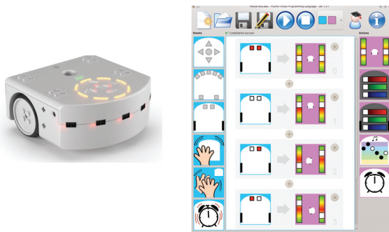
Fig. 1. The Thymio II robot (left) and a screenshot of the VPL programming environment for children (right).
